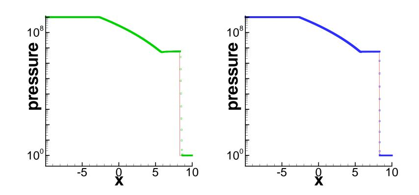
Figure 11: Leblanc problem. T = 0.0001. Left: N = 800. Right: N = 6400. The solid line is the exact solution. Symbols are numerical solutions.  $\Delta x = \frac{20}{N}$  with the positivity limiter. log-scale of pressure.
