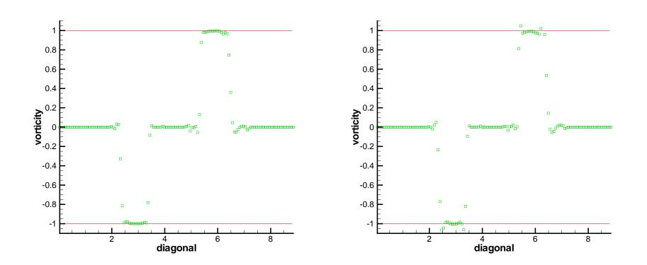
Figure 2: Vorticity at t = 10,  $P^2$ . Cut along the diagonal.  $128^2$  mesh. Left: with limiter; Right: without limiter.
