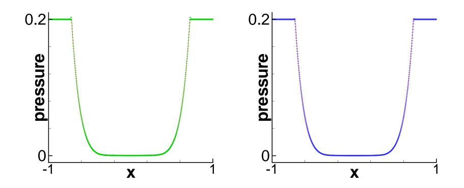
Figure 8: Double rarefaction problem. T=0.6. Left: 1D problem. Right: Cut at y = 0 for the 2D problem. Every fourth cell is plotted. The solid line is the exact solution. Symbols are numerical solutions.  $\Delta x = \frac{2}{N}$ , N = 800 with the positivity limiter. Pressure.
