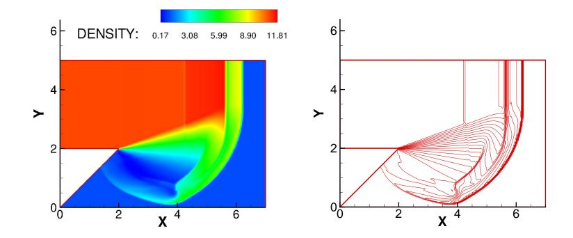
Figure 16: Density. Detonation diffraction at a  $135^{\circ}$  corner.
