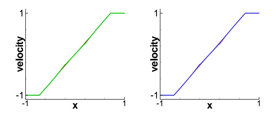
Figure 9: Double rarefaction problem. T=0.6. Left: 1D problem. Right: Cut at y = 0 for the 2D problem. Every fourth cell is plotted. The solid line is the exact solution. Symbols are numerical solutions.  $\Delta x = \frac{2}{N}$ , N = 800 with the positivity limiter. Velocity.
