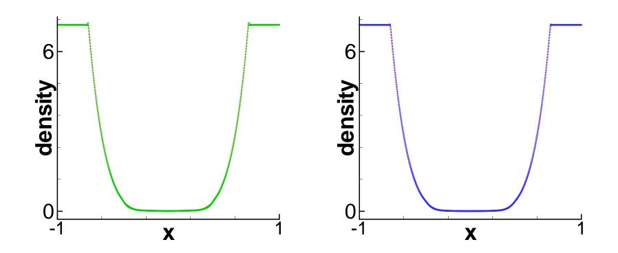
Figure 7: Double rarefaction problem. T=0.6. Left: 1D problem. Right: Cut at y = 0 for the 2D problem. Every fourth cell is plotted. The solid line is the exact solution. Symbols are numerical solutions.  $\Delta x = \frac{2}{N}$ , N = 800 with the positivity limiter. Density.
