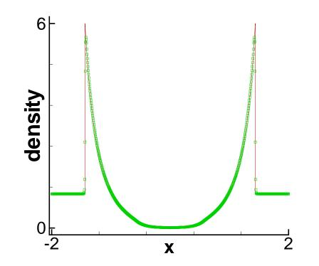
Figure 4: 1D Sedov blast. The solid line is the exact solution. Symbols are numerical solutions. T = 0.001. N = 800.  $\Delta x = \frac{4}{N}$ . TVB limiter parameters  $(M_1, M_2, M_3) = (15000, 20000, 15000)$ . Density.
