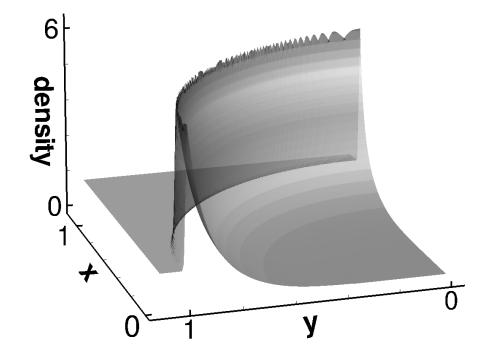
Figure 6: 2D Sedov blast, plot of density. T = 1. N = 160.  $\Delta x = \Delta y = \frac{1.1}{N}$ . TVB limiter parameters  $(M_1, M_2, M_3, M_4) = (8000, 16000, 16000, 8000)$ .
